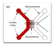
In view of applications, we then want to design integrated systems via nano / micro fabrication techniques (oxides deposition, microfluidics, photolithography, electron microscopy, AFM ...). One of the limiting steps concerns the integration of electrodes within a microchannel. To achieve this goal, we propose an innovative approach based on sub-micrometric gold colloids.
